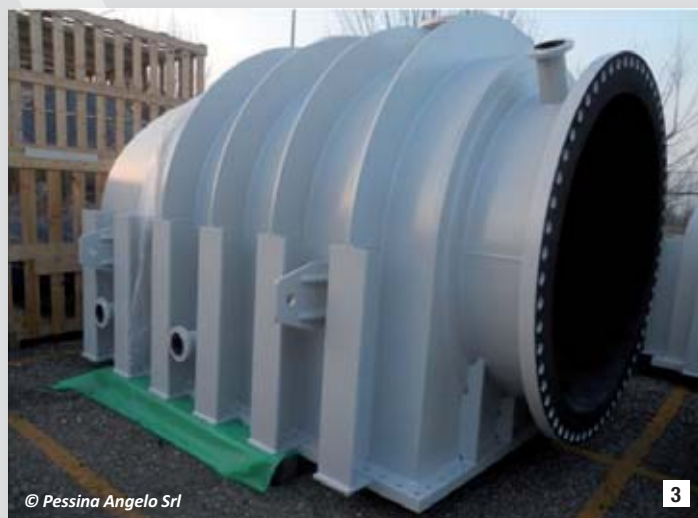
A heat exchanger head with inner lining in polychloroprenic rubber, a type of synthetic rubber that is particularly resistant to sea water, also used for riser tubes produced for oil platforms and for the cartridge filters for sea water.
