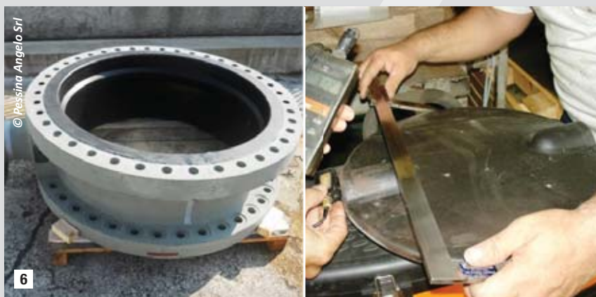
6 EPDM rubber is used to coat cisterns to transport acids, on railways and on wheels. In this photo it is possible to see the lining of bodies and discs of butterfly valves.
