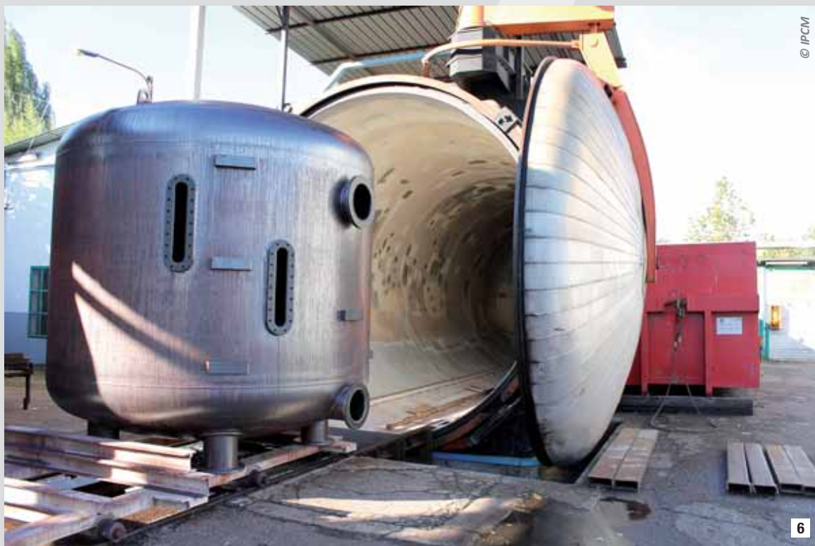
6 A filter exiting the autoclave after the vulcanisation of the ebonite coating.
