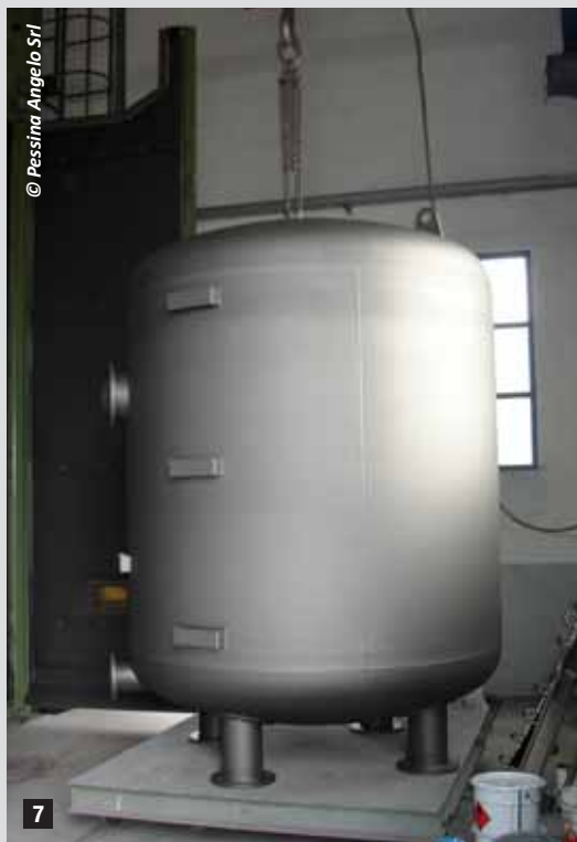
7 After the vulcanisation stage, the filter is again subjected to sandblasting, this time on the outside, in order to be prepared to receive the possible surface finish.
